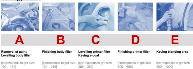
The application and usage of the new Audurra premium abrasives system is easier thanks to the new sanding steps A-B-C-D-E. Only 8 items cover 90% of the applications. The required sanding result is realized with material and cost savings through a clear process with adjusted grit sizes according to application, not according to standards. The simplified process (only 4 grits for paint preparation) avoids application errors and guarantees re-coatability without scratch and swirl marks.
