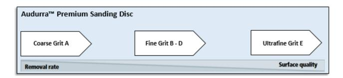
The 15-holes Premium Sanding Disc E is a fine sanding disc with a film backing. The multi-hole Premium Sanding Discs A-D are manufactured with a paper backing. Analog to the abrasives range available from competition Axalta decided on launching the premium sanding disc E with standard 15-hole pattern. Multi-hole discs have a clear advantage when sanding putties and fillers up to grit P600. As of P800 and finer this advantage gets lost.
