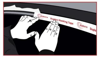
Remove the film liner from the wide section of tape, pull down and mask off the rubber seal.
