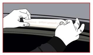
Remove the liner from the narrow section of tape and stick it to the underside of the roof rail and repeat.
