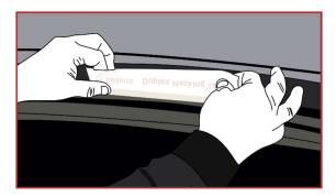
Remove the liner from the narrow section of tape and stick it to the underside of the roof rail and repeat.
