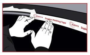
Remove the film liner from the wide section of tape, pull down and mask off the rubber seal.
